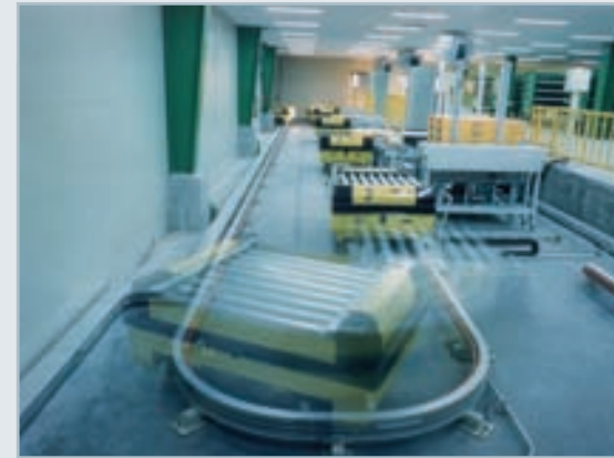
● RTV (Robotic Transfer Vehicle)
